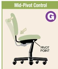
**G** Allows user to recline at a more natural angle than the traditional tilt control. "Pivot point of chair is positioned slightly forward" toward the front of the seat.
