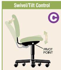
**C** Places the "pivot point directly above the base center" and allows the user to lean back in a seated position.
