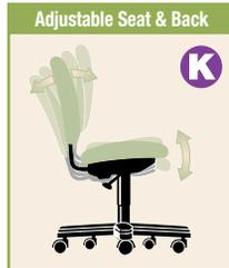
**K** Allows user to "adjust and lock seat and back angle" of chair independently of each other.
