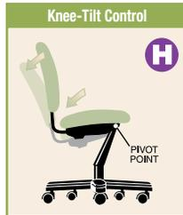
**H** Allows user to fully recline while keeping feet comfortably on the floor. "Pivot point is placed near the front of the seat."
