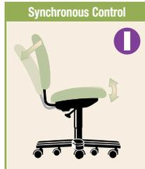
**I** Automatically "adjusts seat and back angle while maintaining a 2:1 recline ratio", providing optimum back support and minimal seat rise.
